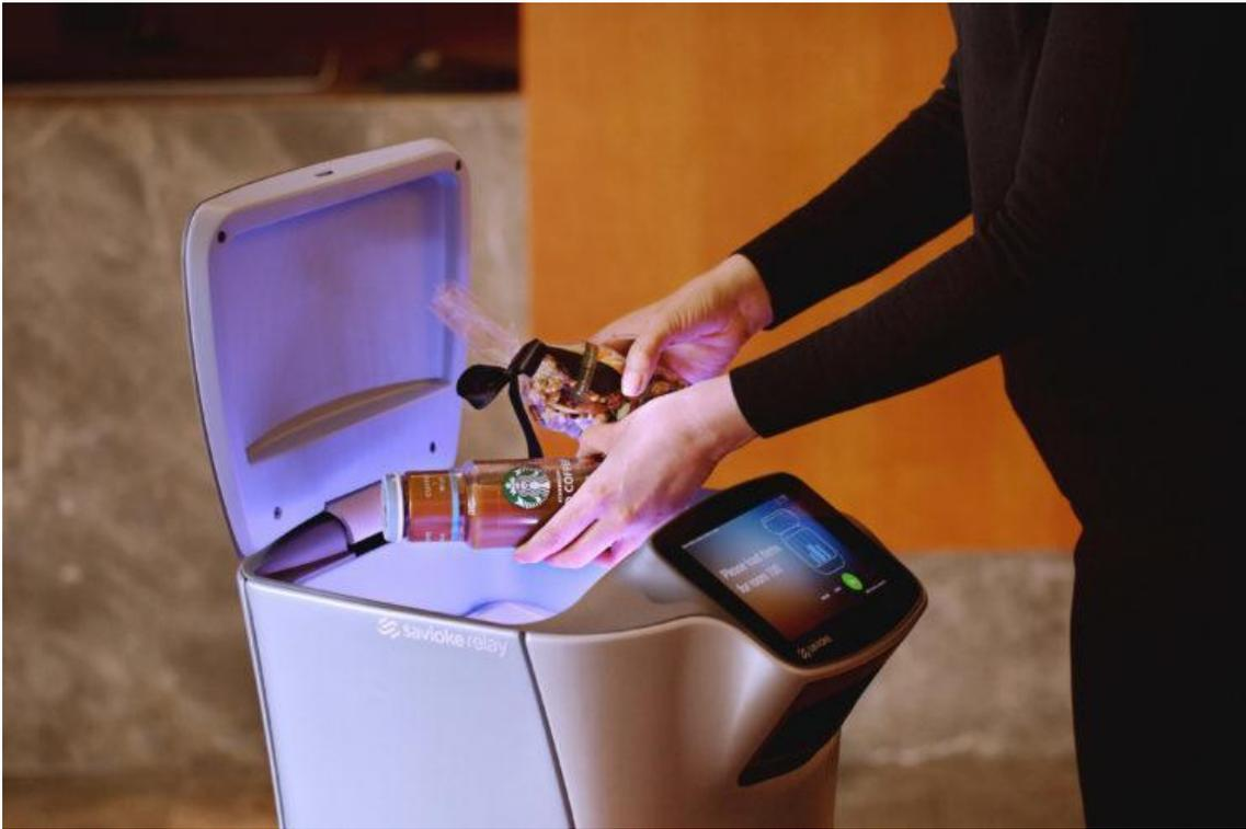
*Savioke's Relay robot being loaded*
